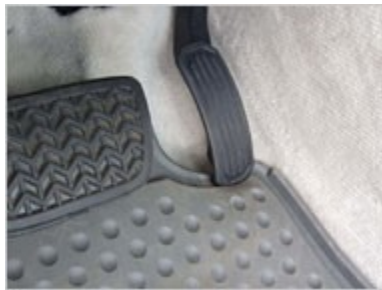
The accelerator of a Lexus stuck on a floor mat.
