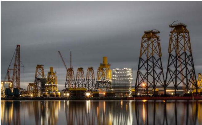
Beatrice OFW Jackets at Smulders Fabrication Yard before transportation to Nigg
