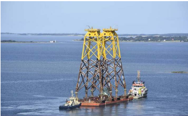
Transport of Beatrice OFW Jackets to Field on Cargo Barge with two Tugs
