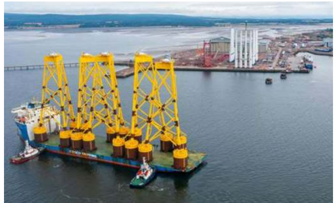
Xiang Yun Kou (XYK) delivering the first five Seagreen jackets from the fabrication yard in Jutal, China to Nigg, Cromarty Firth, Global Energy Group
