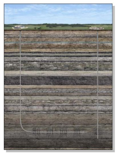
Horizontal and Vertical Well Completions Source: DOE, Fracing Primer
