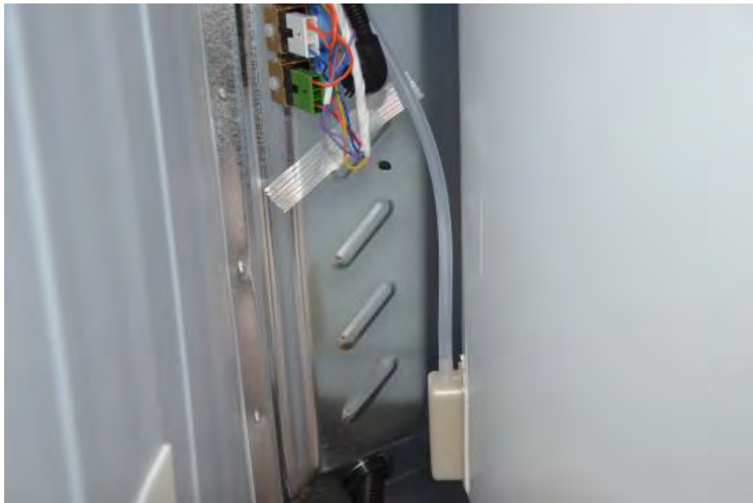
Figure 8 – Variations in placement of the strain relief tap in exemplar washing machines model # FAHE4044MW (Top), and model # FFLG2022MW (Bottom)
