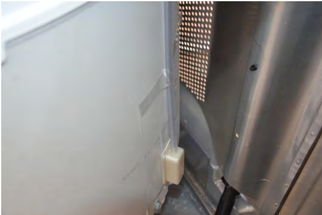
Figure 9 – Variations in placement of the strain relief tap in exemplar washing machines model # FFLE2022MW (Top), and model # FEX831S (Bottom)
