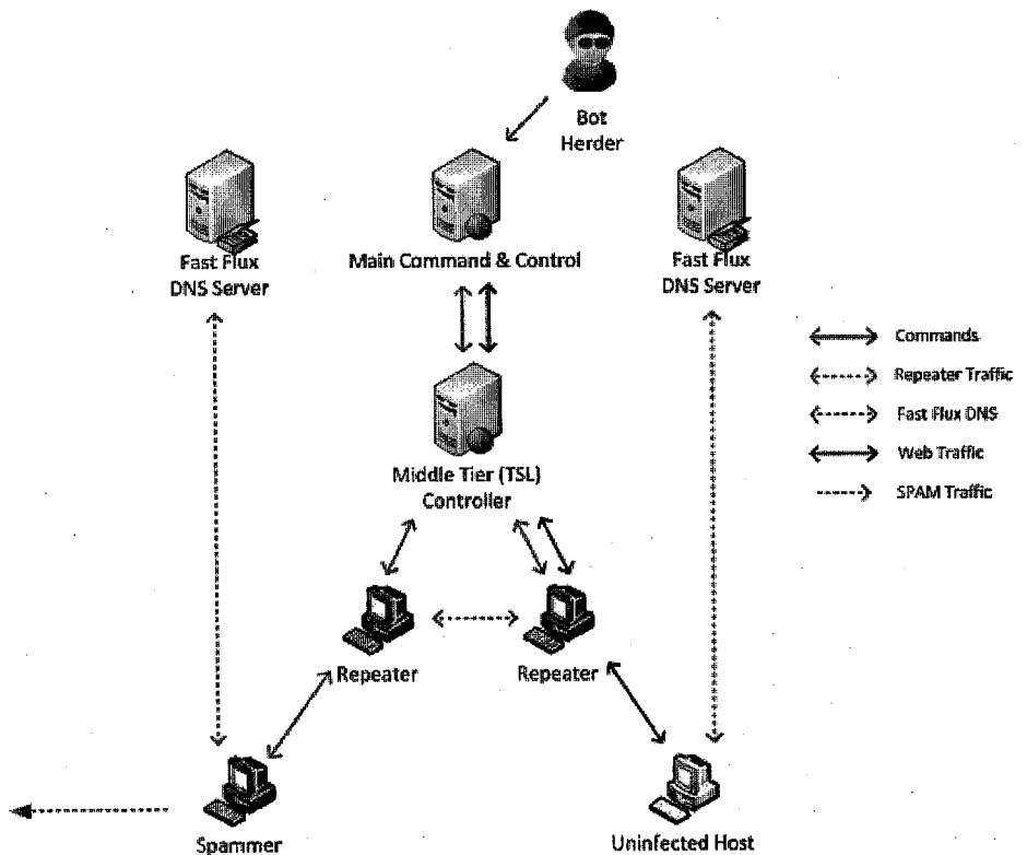
26. The lowest “Spammer Node” tier in this architecture is made up of infected user computers that have been determined to be behind firewalls or otherwise not directly accessible from the Internet. The botnet software placed on these infected computers sends, without the user’s knowledge or permission, unsolicited bulk email (often known as “spam”). This spam
