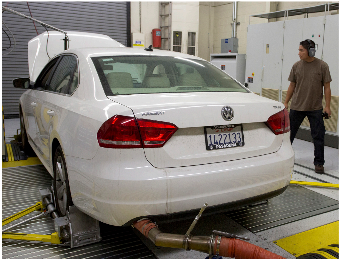
The California Air Resources Board's Arie Jan Haagen-Smit Laboratory, where emissions from thousands of cars, motorcycles and other vehicles are tested each year, in El Monte, Calif., Sept. 25, 2015. | New York Times News Service
